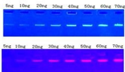
1. Sensitivity detection of DSView™ under UV transmission(wave length 300nm)
